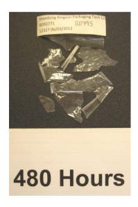
Following its ageing process of 480 accelerated ageing hours (calculated to around 10.5 months at 20°C) the clear POF shrink film sample can be seen to have lost its significant physical properties, is exhibiting extreme friability, and breaking up when handled.
